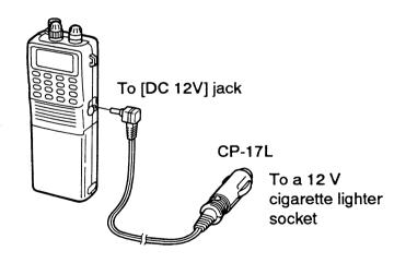
The OPC-515L DC POWER CABLE with a 12 V DC power supply can be used instead of the CP-17L.
