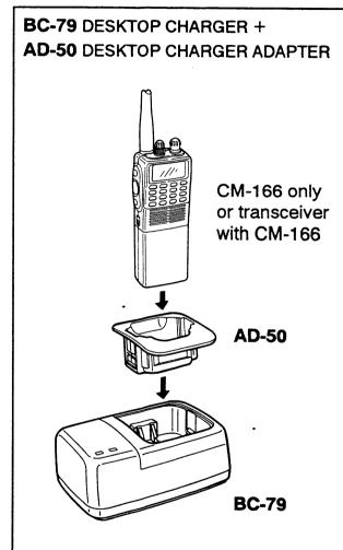
Rapidly charges the CM-166 in approx. 1.5 hrs. An AC adapter is packed with the BC-79. An optional CP-13/L or OPC-288/L can be used instead of the supplied AC adapter.
